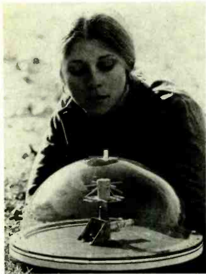
A HALF-WAVE ANTENNA ON 3 GHz, this 4-inch high antenna will be the link to Earth for the NASA Lander due to touch down on Mars July 4, 1976. The Earthling studying it is RCA secretary Carol Safford.
